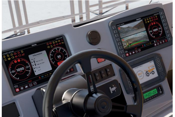
Connectivity is extremely important across the industry and the **DSEM812** offers GPS and Wi-Fi connectivity. Built-in Wi-Fi on machinery equipment provides a range of options for service personnel and machine operators to take advantage of. Large amounts of data can be collected from multiple locations on a machine and passed via CANbus or Ethernet to the **DSEM812** display, where data can be accessed wirelessly.
