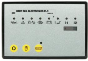
The DSE703 is an Automatic Start Control Module that offers an excellent range of engine monitoring and protection features. The module has been designed to monitor over speed, under speed, high engine temperature, low oil pressure, battery charge fail and fail to start.
