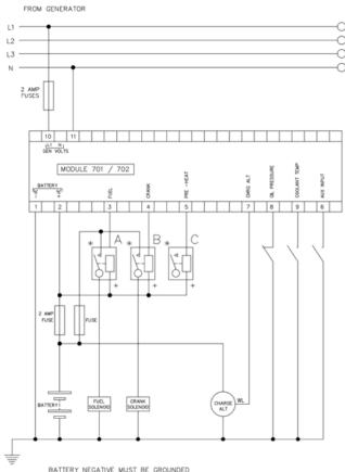
TERMINALS SUITABLE FOR 22-16 AWG (0.6mm<sup>2</sup> - 1.3mm<sup>2</sup>) FIELD WIRING TIGHTENING TORQUE = 0.8Nm (7lb-in)
