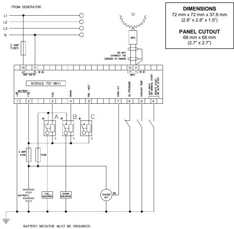
TERMINALS SUITABLE FOR 22-16 AWG ( $0.6mm^2 - 1.3mm^2$ ) FIELD WIRING TIGHTENING TORQUE = 0.8Nm (7lb-in)
