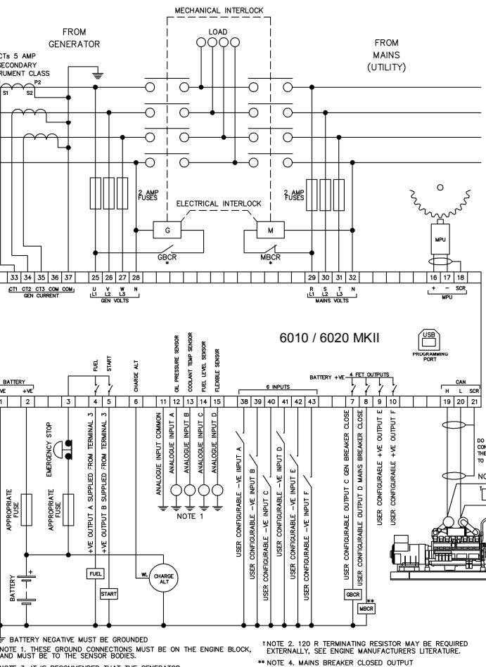
**NOTE:** A larger version of the typical wiring diagram is included in the products operator manual. Refer to DSE Publication: 057-218 DSE6010 MKII & DSE6020 MKII Operators Manual
