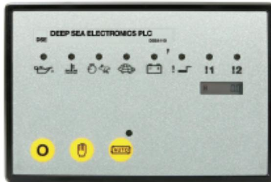
The DSE703 is an Automatic Start Control Module that offers an excellent range of engine monitoring and protection features. The module has been designed to monitor over speed, under speed, high engine temperature, low oil pressure, battery charge fail and fail to start.
