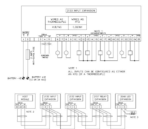
NOTE 2 AS A TERMINATING RESISTER IS INTERNALLY FITTED TO THE HOST CONTROLLER, THE HOST CONTROLLER, MUST BE THE FIRST UNIT ON THE DSEnct NOTE 3 A 120 DHM TERMINATION RESISTOR MUST BE FITTED TO THE LAST UNIT ON THE DSEnet
