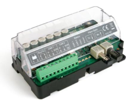
The DSE124 is a CANbus extender capable of extending either the Multiset Comms (MSC) Load Share Link or engine CANbus.
