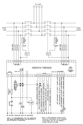
NOTE: Terminals 8, 9, 25, 26, 27 and 28 are fitted to DSE4220 only. For DSE4210, Gen Breaker Close is set to Output C (terminal 6).
