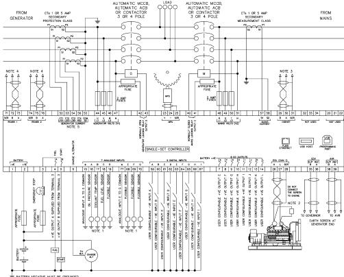
NOTE 1. THESE GROUND CONNECTIONS MUST BE ON THE ENGINE BLOCK, AND MUST BE TO THE SENSOR BODIES.
