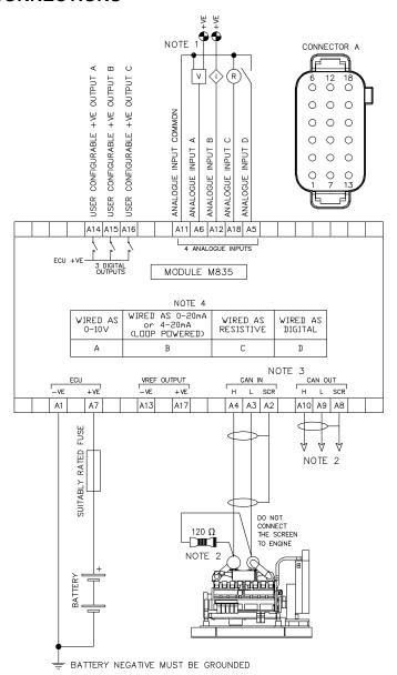
NOTE 1. ANALOGUE INPUT COMMON MUST NOT BE GROUNDED, IT IS LINKED INTERNALLY TO TERMINAL A1.
