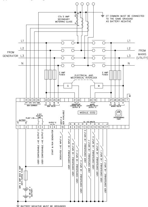
TERMINALS SUITABLE FOR 22-16 AWG (0.6mm - 1.3mm ) FIELD WIRING TIGHTENING TORQUE = 0.8Nm (7lb-in)
